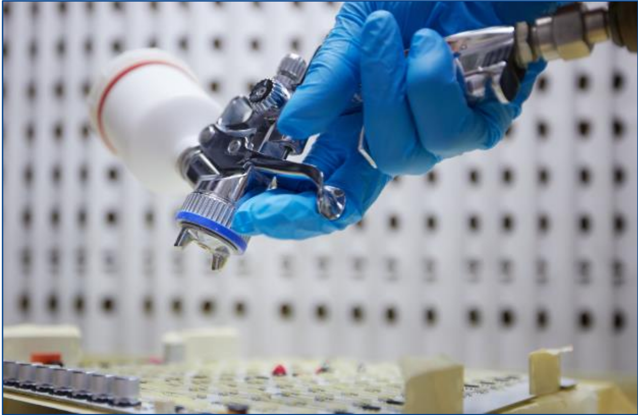
manual painting with a wide variety of paints from the manufacturers Peters Lacke, Humiseal and Henkel
