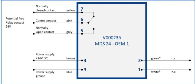
\* The contacts for the Hall generator are not connected in version V000235 (MDS 24 - OEM 1)
