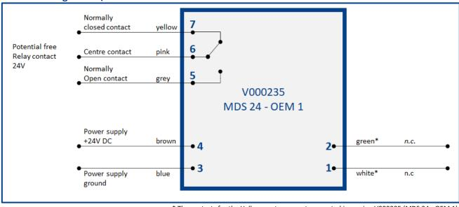
$<sup>^{*}</sup>$  The contacts for the Hall generator are not connected in version V000235 (MDS 24 - OEM 1)
